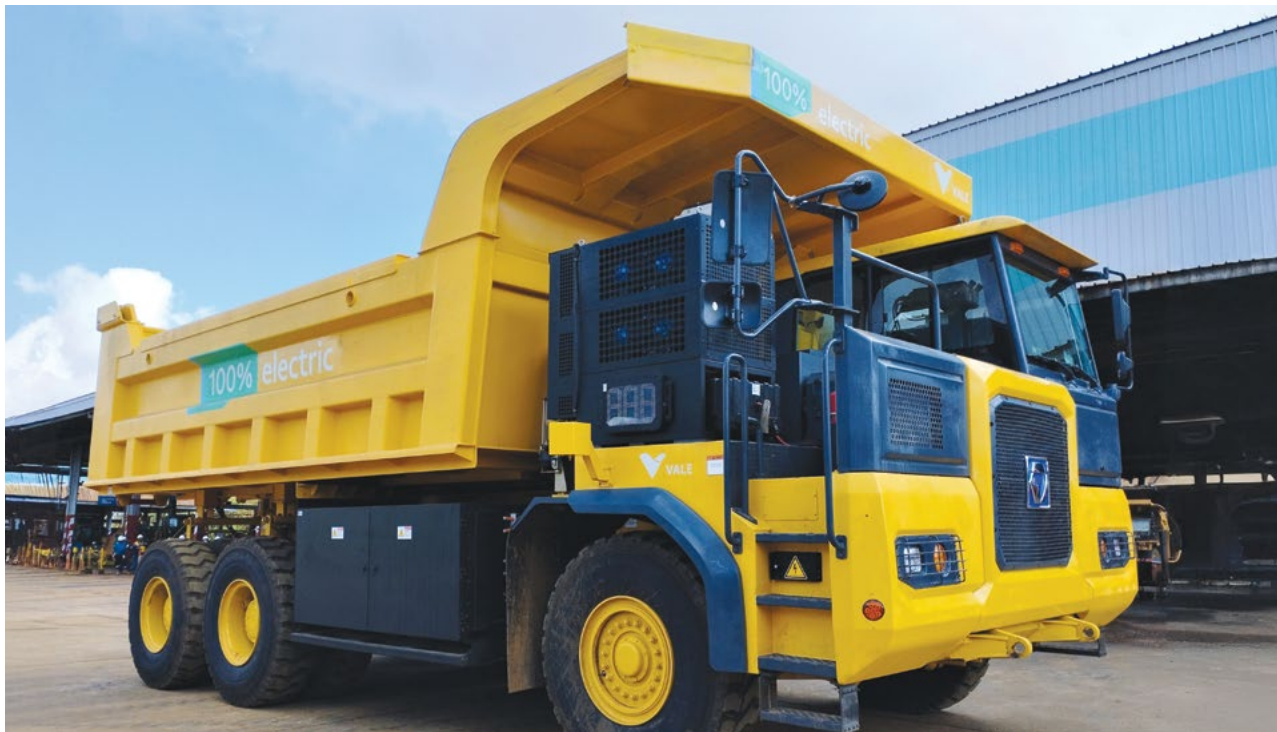
Electric-powered haul truck, used to transport mining material in Indonesia. Photo via Shutterstock.
